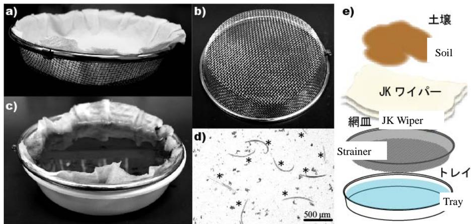
Fig. Example of Baermann tray: a) Strainer set with JK Wiper<sup>®</sup>, b) Strainer (bottom view), c) Nematode extraction, d) Extracted nematodes (\*), e) Pattern diagram.
