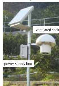
An automated air temperature data acquisition system
