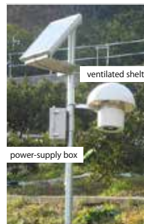
An automated air temperature data acquisition system
