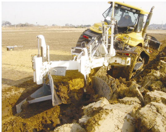
Fig.21 深さ1mの反転が可能なプラウ Prau that can reverse depth of 1m
