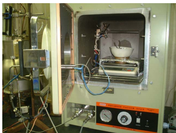
Photo Overview of furnace used for biomass burning experiments.
