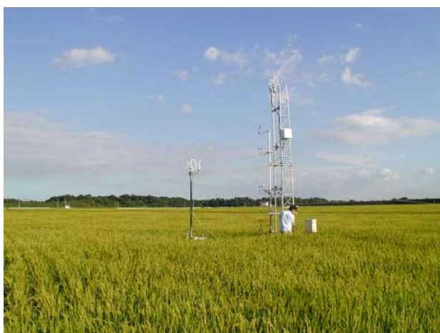
Photo 1 The flux site at Mase, near Tsukuba in central Japan, in August. Carbon dioxide exchange between a single-cropping rice paddy field and the atmosphere is continuously monitored at this site.
