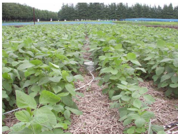
Photo 1 Soil respiration chamber placed among soybeans under no-tillage cultivation.
