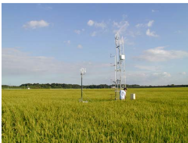
Photo 1 The flux site at Mase, near Tsukuba in central Japan, in August. Carbon dioxide exchange between a single-cropping rice paddy field and the atmosphere is continuously monitored at this site.
