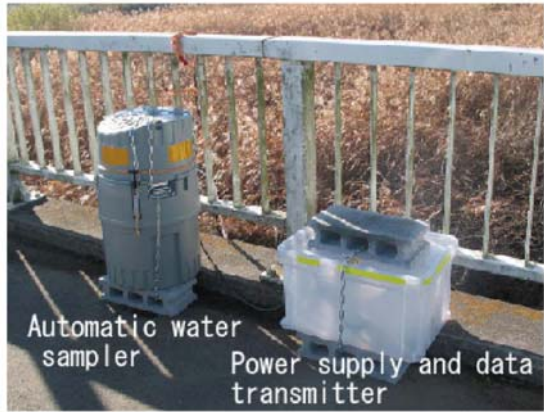
Fig. 2 Water quality monitoring using an automatic water sampler (IV-3)
