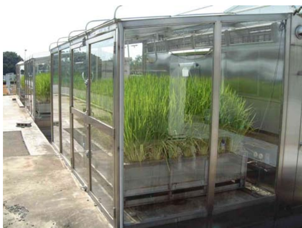
Fig. 1 Naturally sunlit controlled-environment chambers at the National Institute for Agro-Environmental Sciences. Here it is possible to investigate plant response, canopy photosynthesis and respiration rates, and other things under natural sunlight conditions with controlling the air temperature, humidity, and CO 2 concentration inside the chamber.
