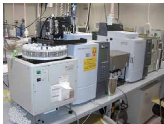
Fig. 1 Overview of the automated three-greenhouse-gas analyzer.
