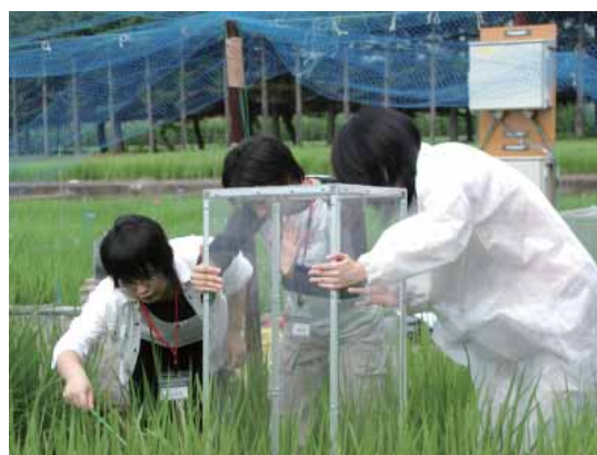
Photo 2 Setting up greenhouse gas monitoring apparatus in a paddy field
