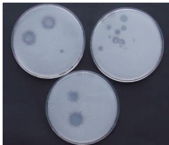
Fig. 1 Selection of molds that decompose biodegradable plastic. Colonies of molds that decompose biodegradable plastic are surrounded by the transparent area .
