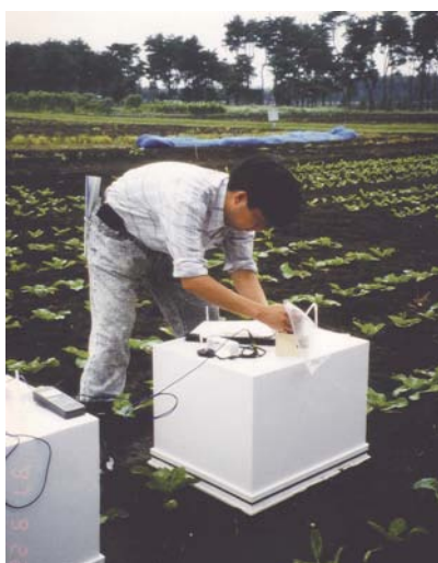
Photo 1 Researcher performing manual sampling. The manual sampling method, which has been used primarily until now, requires that people do everything from installing the chamber to taking samples, and therefore was labor-intensive.
