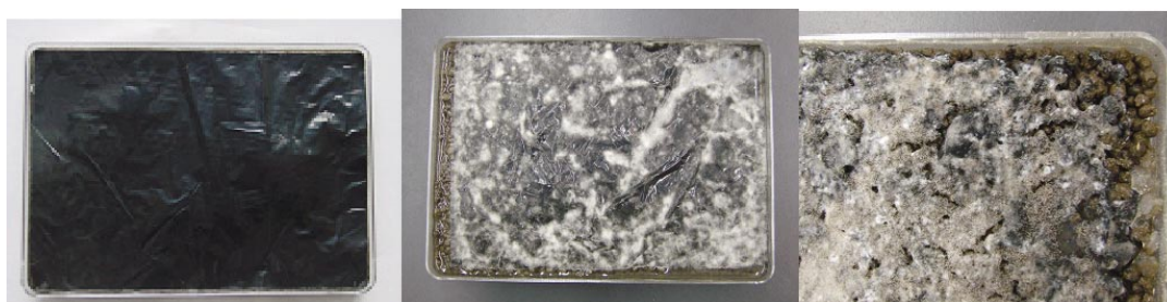
Fig. 3 Decomposition of biodegradable plastic film (PBSA) placed over potting soil by application of the enzyme produced by strain 47-9.
