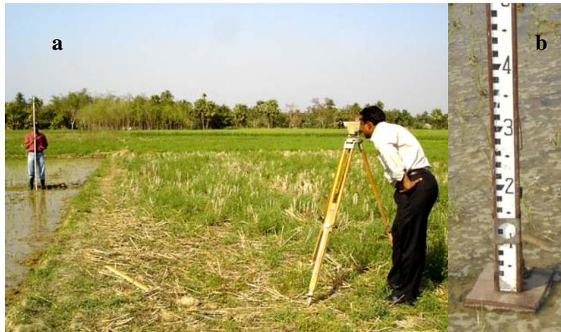
Fig. 2a, b. Measuring elevation using Theodolite (left) and Staff (right)
