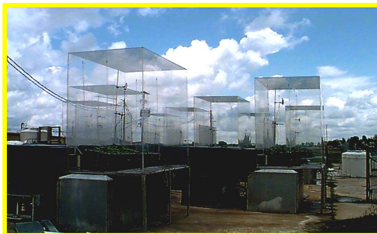
Fig. 2. The Soil-Plant-Atmosphere-Research (SPAR) chambers at Starkville, Mississippi, USA. The SPAR facilities in Florida, Maryland, and Mississippi have been influential in US research concerning the effects of high temperatures and other climate change factors on crop production.
