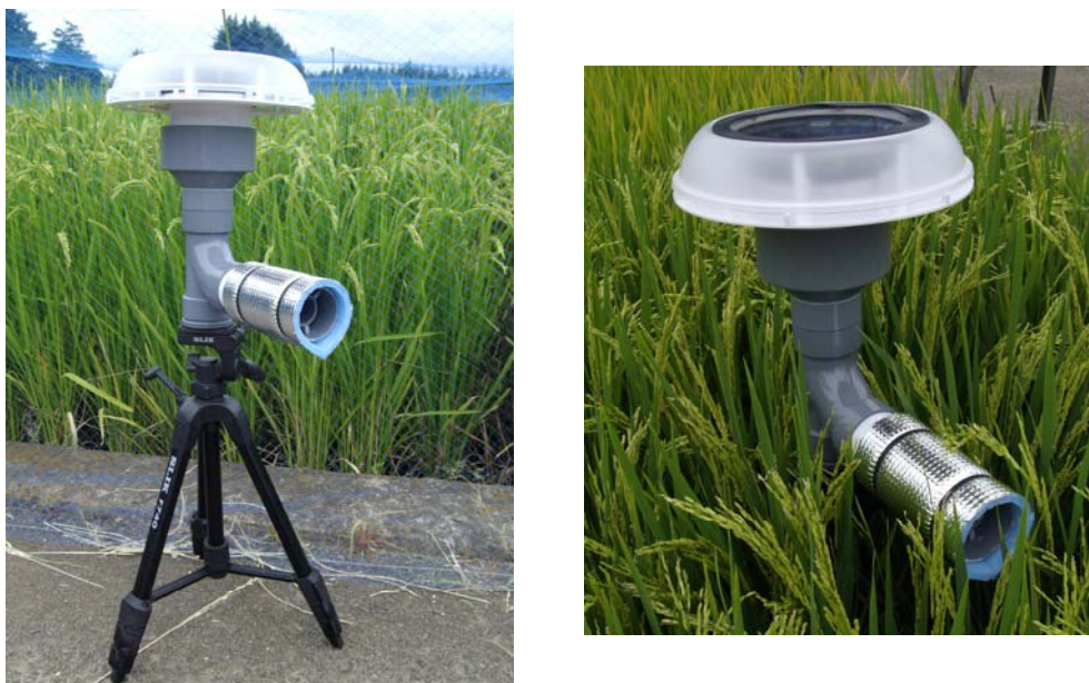
Fig. 1. Prototype of the temperature and humidity profile measurement system equipped with a force-ventilated radiation shield and a solar panel.
