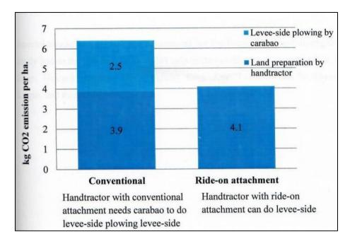
Fig. 3. Emission from handtractor with conventional and ride-on attachment.
