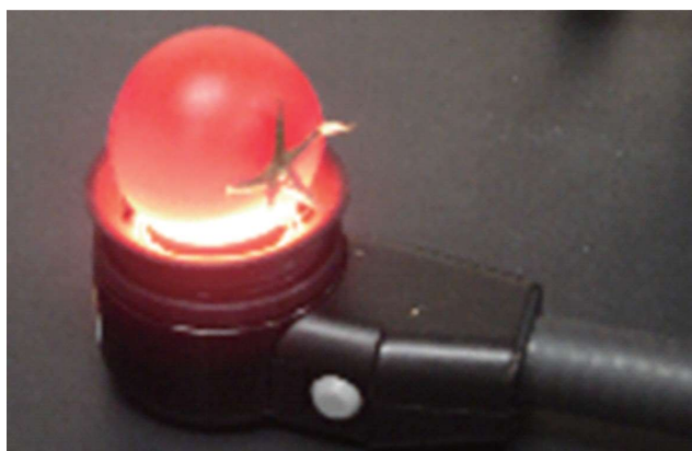
Nondestructive and noncontact measurement of tomato using diffuse reflected light
