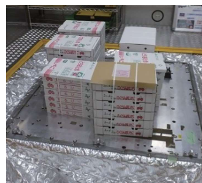
Three-dimensional vibration simulator that enables reproduction of transportation vibration
