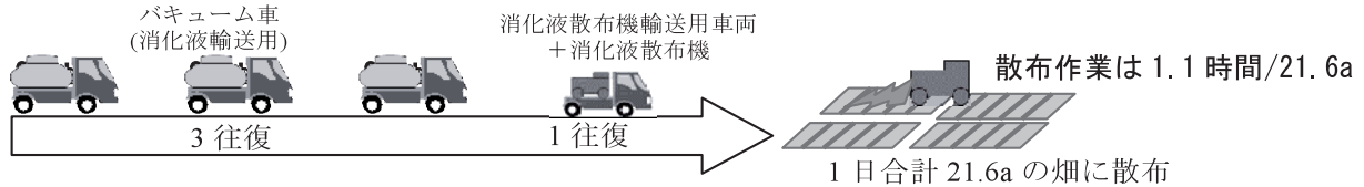
Fig.17 畑への消化液の輸送・散布のシナリオ条件 (シナリオ 3) Scenario of digested liquid transportation and application to upland field (Scenario 3)
