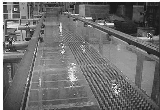
Photo 3-2 模擬水没植生を設置した水路の概要 Outline view of experimental flume where simulated submerged vegetation was set up
